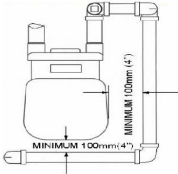
Figure 3 Minimum Spacing Requirements to Adjacent Piping
